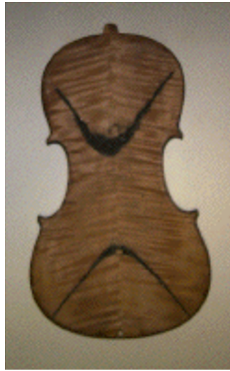
Figure 5.10: Chladni pattern found for a violin, which resembles the nodal lines found in our simulation. VIII
